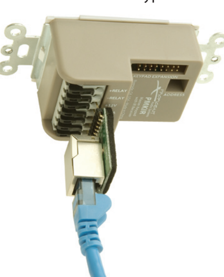
Figure 9 RJ45 Attached to Keypad and CAT5
